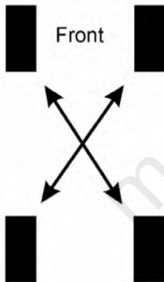
Fig. 2: Popular Tire Rotation Patterns - Without Dual Rear Wheels
